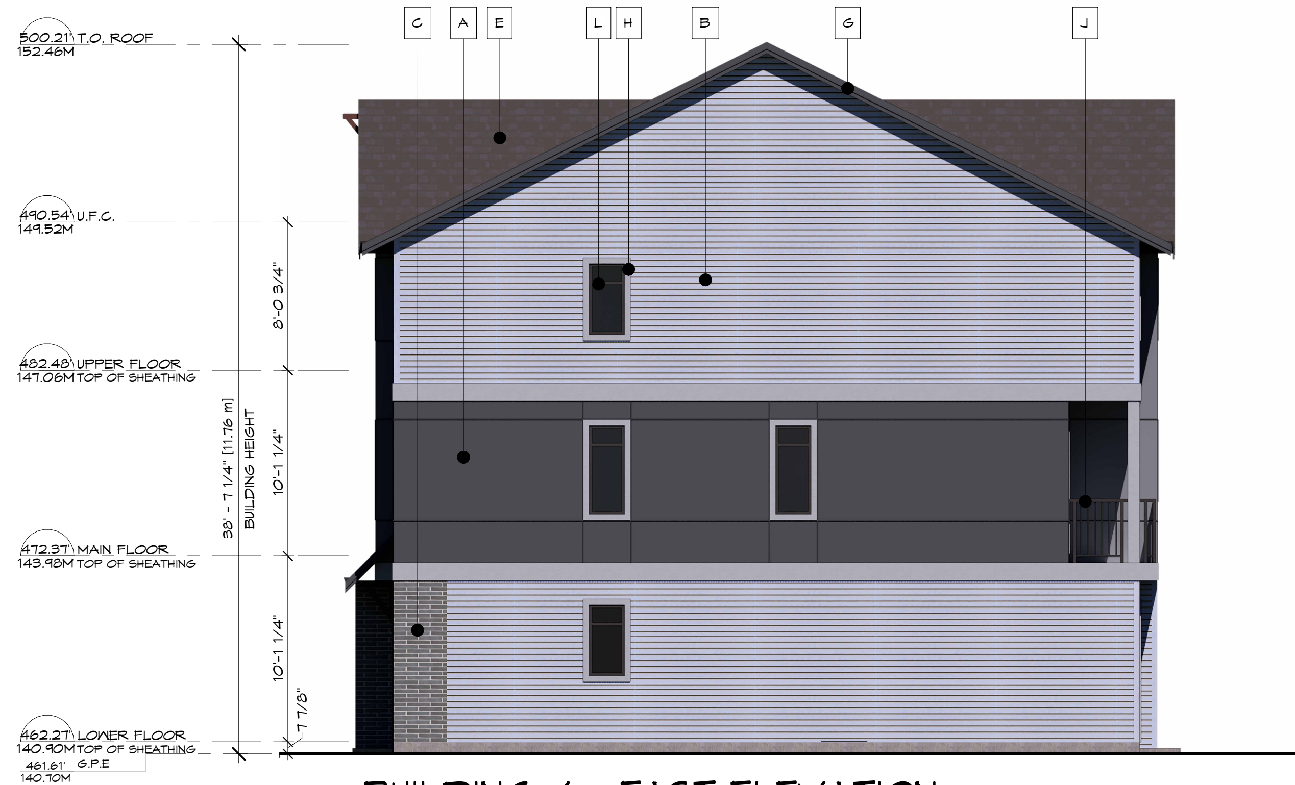
2 BUILDING 4 - EAST ELEVATION A-4.5 3/16" = 1'-0"
