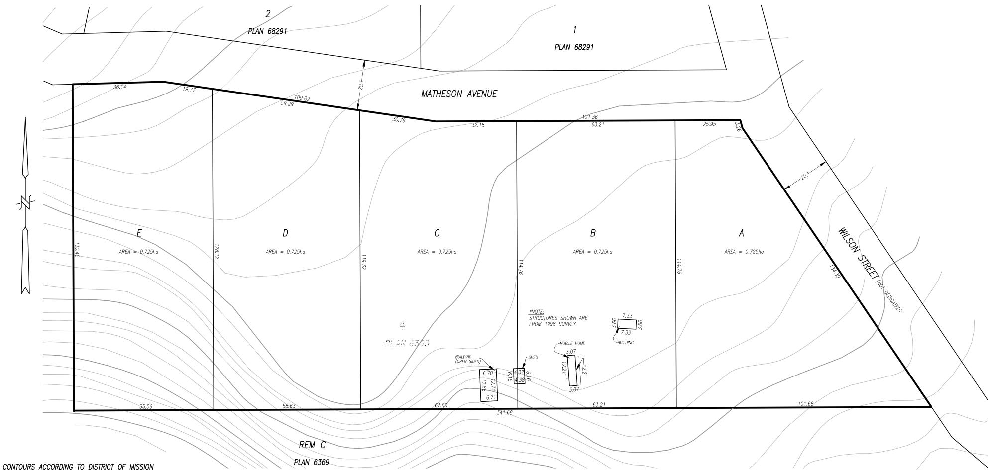
INFORMATION REGARDING TOPOGRAPHY AND UNDERGROUND SERVICES IS COMPILED FROM FIELD SURVEY AND SERVICE LOCATION PLANS. ALL U/G SERVICE LOCATIONS ARE APPROXIMATE AND MUST BE CONFIRMED BY THE USE OF PIPE LOCATOR (M-SCOPE) AND MANUAL DIGGING.
